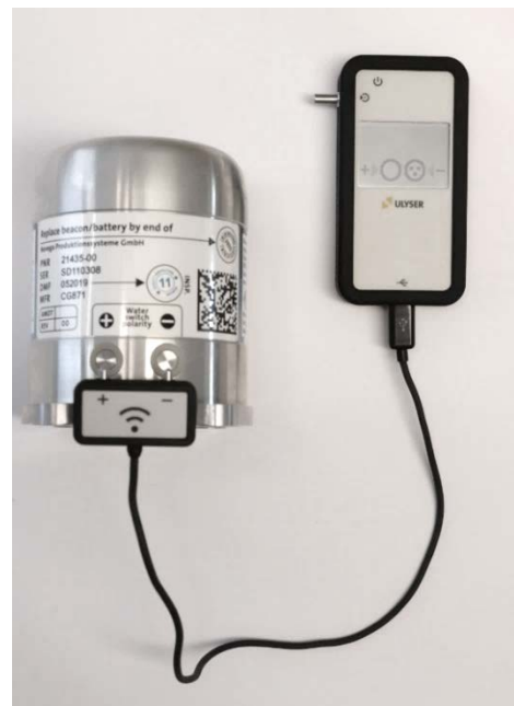
Figure 27: Functional Test with an example LF-ULD
