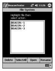
Tapping a file name will select the file name. Tapping the file name again will de-select it. Pressing **Select All** will select all of the files. The **Open** and **Rename** buttons will only work when a single file name has been selected. To delete multiple files, tap **Select All** or select each file individually, then press **Delete**.
