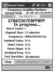
In the measurement folder on the PDA, a delimited text file is created. This text file is updated after each burst during the stability measurement test. This delimited text file can be imported to your favourite spreadsheet or database application.
