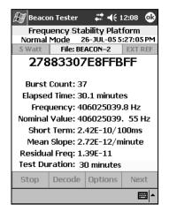
• Once Test Duration has been reached, one final burst is automatically captured to create the Test Report.
