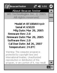
This screen displays information about the Beacon Tester card installed in the PDA, along with the Firmware and Software dates and versions. The Calibration Due date is shown. A real-time temperature sensor displays the temperature inside the Beacon Tester.
