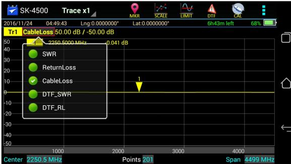
3. Set the frequency start and stop to a range that is greater than the normal range of the antenna.
