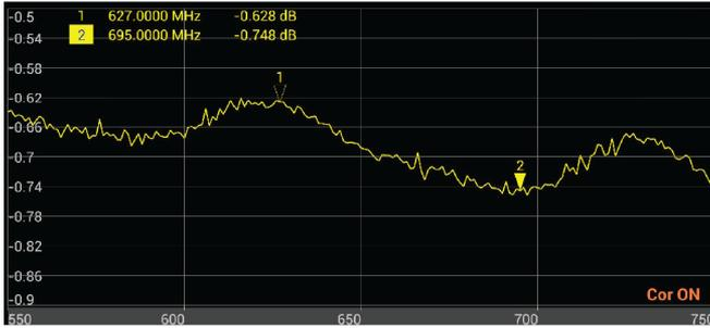
1. Marker 1 and Marker 2 indicate the minimum and maximum loss for the cable under test.
