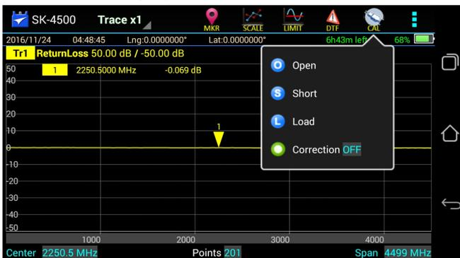
Match measurement verifies and monitors the match conditions in the antenna system at various frequencies. The results are shown on an x-y graph. Frequency is shown on the x-axis and Return Loss or SWR is shown on the y-axis.
