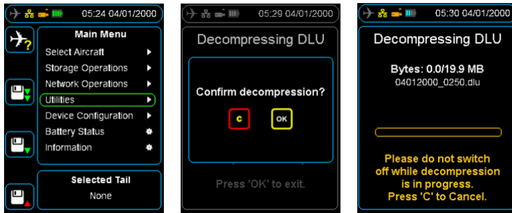
Figure 22 Decompressing Honeywell CVR file away from the aircraft
