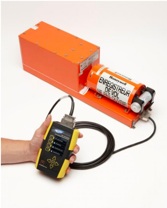
Figure 10 Connecting the HHMPI to the FDR or CVR
