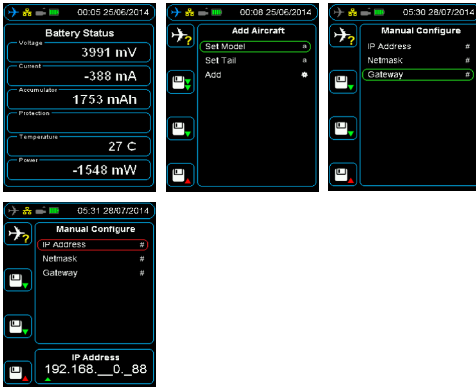
Figure 31 DHCP or manual IP configuration
