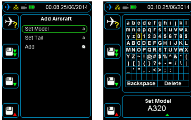
Figure 18 Adding aircraft to the Aircraft List on the HHMPI
