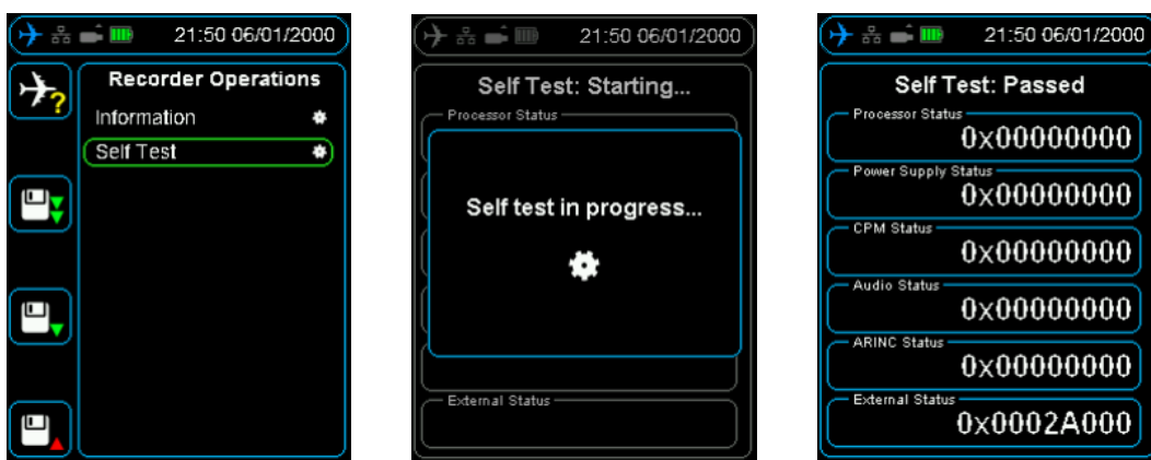
Figure 52 SRVIVR™ Recorder Operations - Self Test
