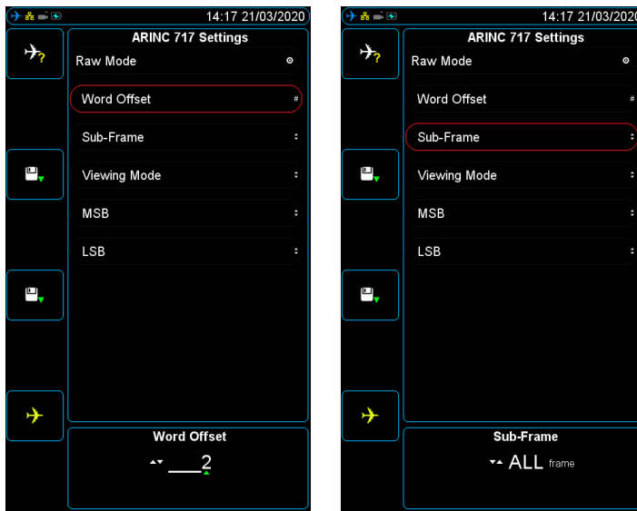
Figure 78 Word Offset and Sub-Frame Selection
