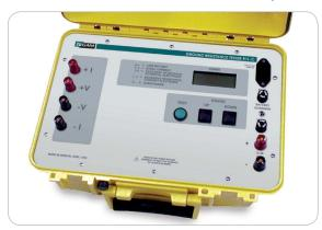
The Model R1L-C is a series of portable ground resistance ohmmeters designed to measure grounding system resistance, as well as soil resistivity, over ranges from milliohms to  $20 \text{K}\Omega$  full scale. The R1L-C is capable of Wenner, Fall of Potential, 62% methods as well as bond and continuity measurements. Two, three and four point measurements are standard for this instrument.
