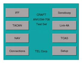
The AN/USM-708 large 4.75" x 3.5" color LCD (NVG compatible) screen and surrounding soft-keys and keyboard provides easy and quick access to a multiple of test screens menus, and display options affording single man operation, instant results, and a host of pre-programmed and manually variable parameters to meet the most demanding requirement's for testing of airborne avionic and communication equipment.
