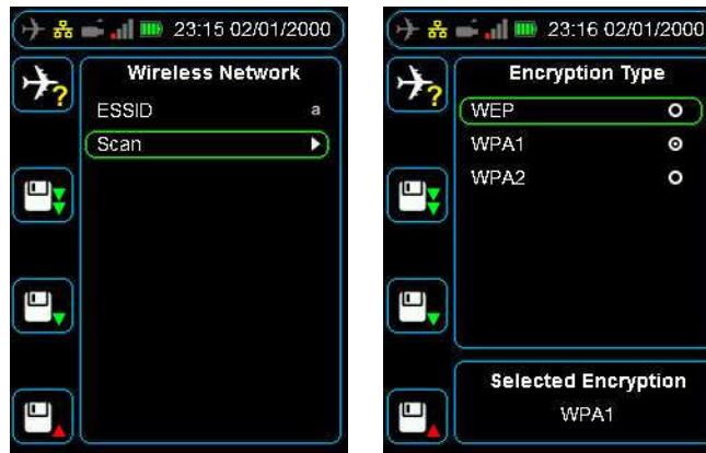
Figure 36.0 Configuring security settings like the encryption type and key
