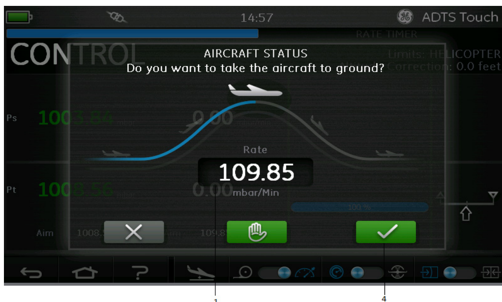
Figure 3-18: Go to ground main screen - Single Channel
