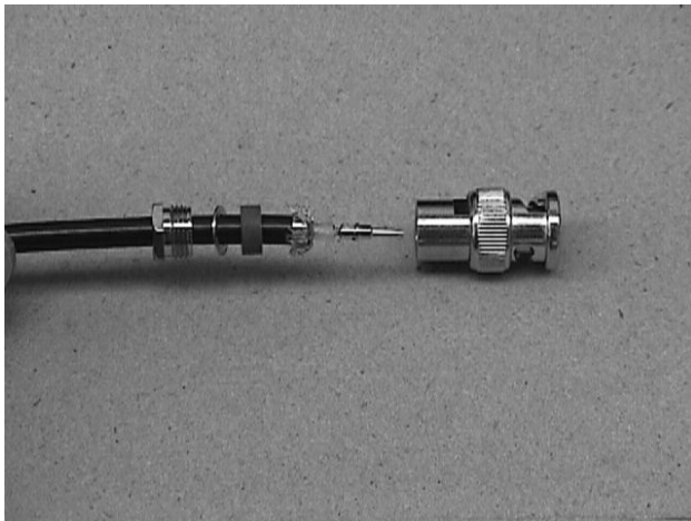
Fig. 3-7. The cable with components in place for final assembly during which the nut at left is screwed into the body at right.
