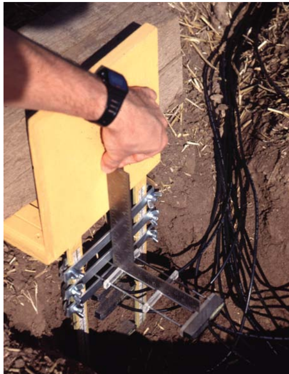
Fig. 4-1. The probe installation jig in use. The square is used to ensure that the probe is horizontal to the soil surface.
